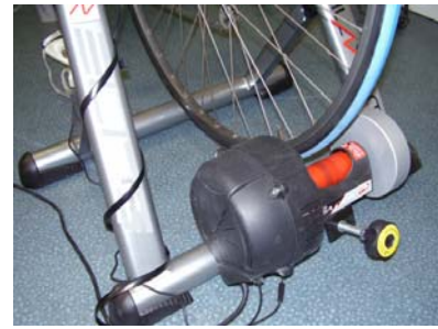
Fig. 2. Photo of the resistance tool (electromagnetic brake), in contact with the rear wheel.
